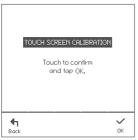
In case that you can't tap any button on the screen correctly, this calibration can adjust the touch screen.
