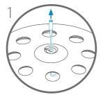
Pass its own cable through the hole and pull it up.
