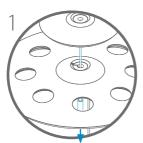
Pass the splash cable through the hole and pull it down.
